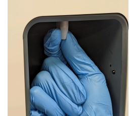
6. Install a new dispensing tip
