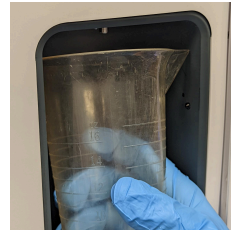
5. Dispense 250mL of water to flush the nozzle
