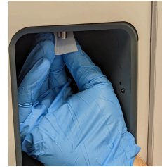
2. Clean the nozzle with an alcohol wipe
