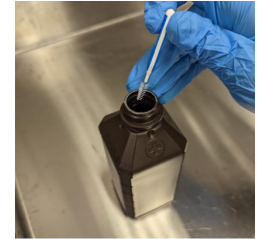
3. Immerse the wire brush in the hydrogen peroxide
