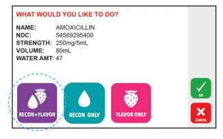
Confirm the info on the screen is correct, make sure you're holding the uncapped medication bottle under the dispensing tip, and press "OK" 4. Select the customer's preferred flavor
